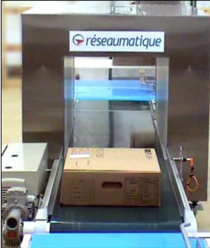
The pilot participants used tunnel readers that Biolog-ID built specifically for the application, in order to read the RFID tags of blood bags inside each box.
