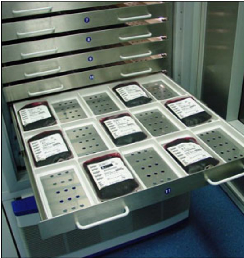
The Biolig-ID Smart Fridge has drawers divided into 15 cells (each storing a single bag), with each cell equipped with a built-in RFID reader antenna to read a bag's RFID tag.
